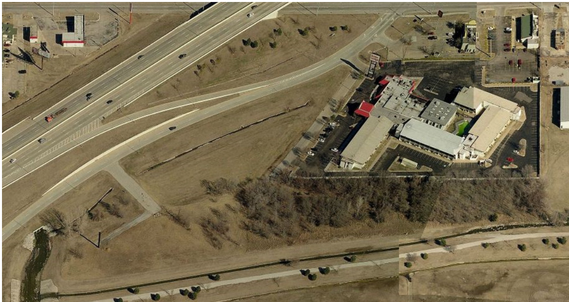
RLA 52 is located southeast of the intersection of E. 11 th St. and I-44, 300 feet north of Tupelo Creek Tributary #4, and 1,000 ft. northeast of the junction of Tributary #4 with Tupelo mainstem. Tributary #4 is in the lower part of the photograph, and Tupelo mainstem in the lower left. During heavy rains, water backs up behind the conduit beneath I-44 into the pocket of low ground to the west of the motel complex.
