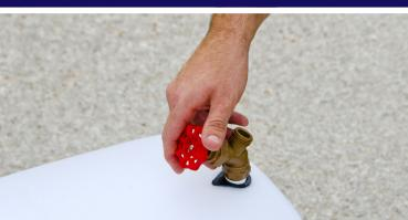
Twist in the threaded end of the faucet into the <sup>3</sup>/<sub>4</sub>" threaded hole of the rubber gasket toward the bottom of the barrel.
