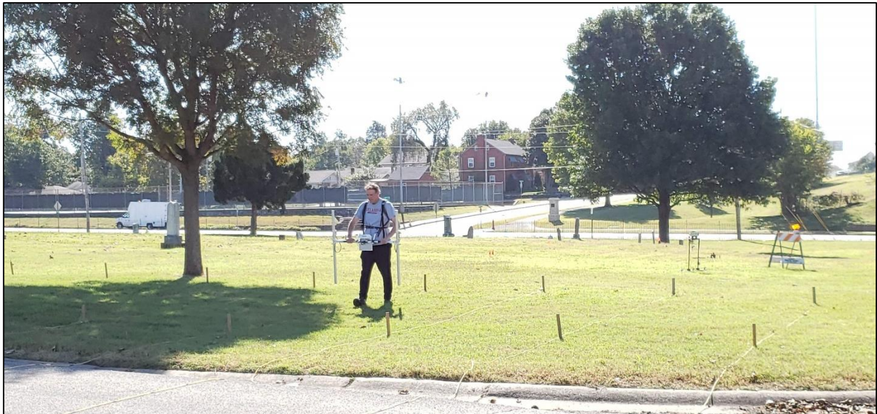
Figure 4. Bartington Grad 601 gradiometer in use at Oaklawn Cemetery. Photo by Angela Berg.
